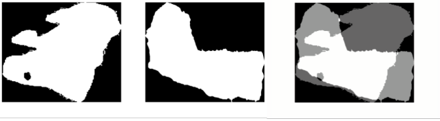
Figure 7. Shape test. On the left two column are segmented images of a candidate fragment pair. On the right are the two segmented fragments on top of one another. It can be visually seen that their Hamming distance corresponds to measuring how well the shapes overlap.
